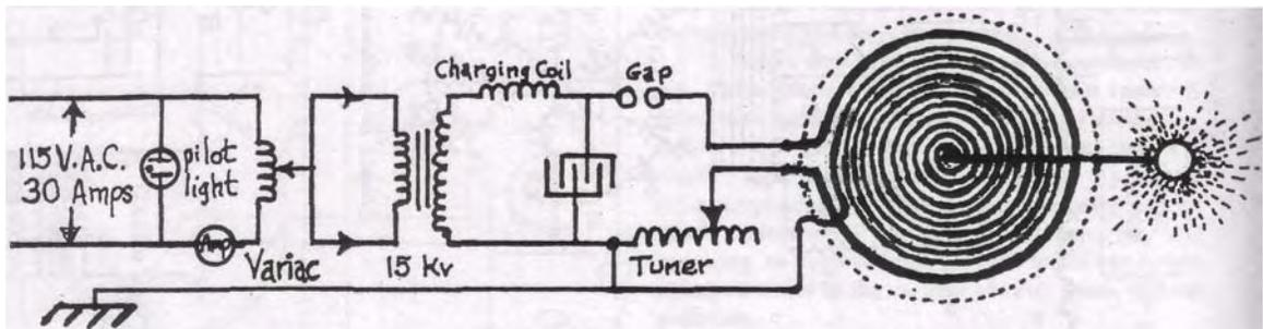
This 150 kv coil design has a single-turn primary and 10-turn secondary (1:10 ratio), with a maximum voltage increase of 15 kv per turn of the secondary. 1/8" increased spacing per turn is sufficient, using a dielectric with a K-value of 4. The secondary wire will be about 1/8" in diameter, and the primary will be a 1/2" wide copper strip about 1/32" thick. The following schedule of spacing between turns is observed:
